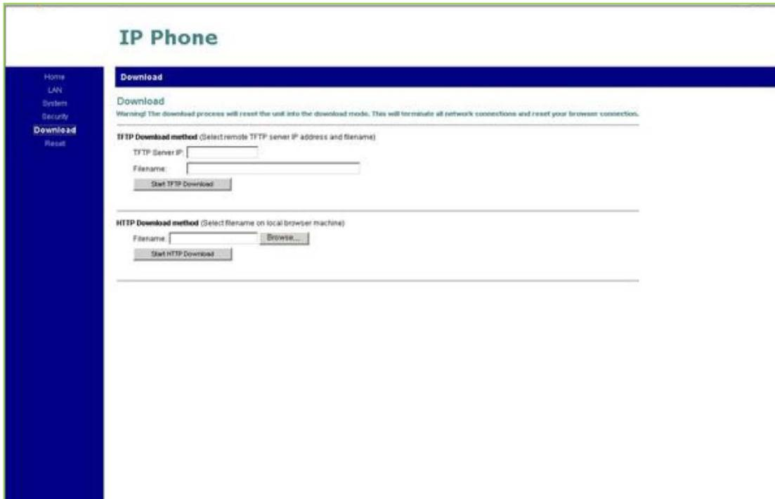
**Figure 7.1.3.2-1 iPECS Phone Direct Connect Upgrade**
